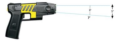
The top probe impacts the target near the laser beam and can vary depending on distance, type of cartridge, etc. See www.TASER.com for current specifications.
