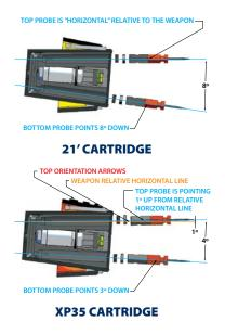
**WARNING:** The XP35 TASER Cartridge is not reversible. It has raised orange arrows printed on the side of the cartridge that is inserted towards the top of the device.
